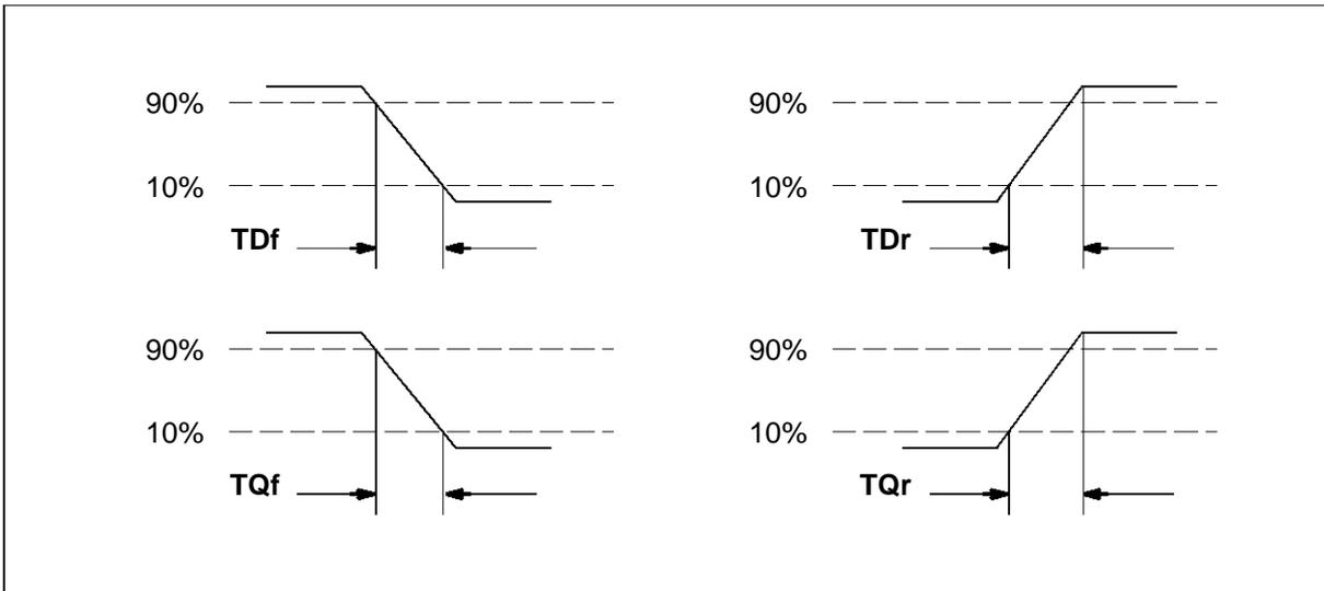
Figure 7.3 IMS C011E input and output edge timing
