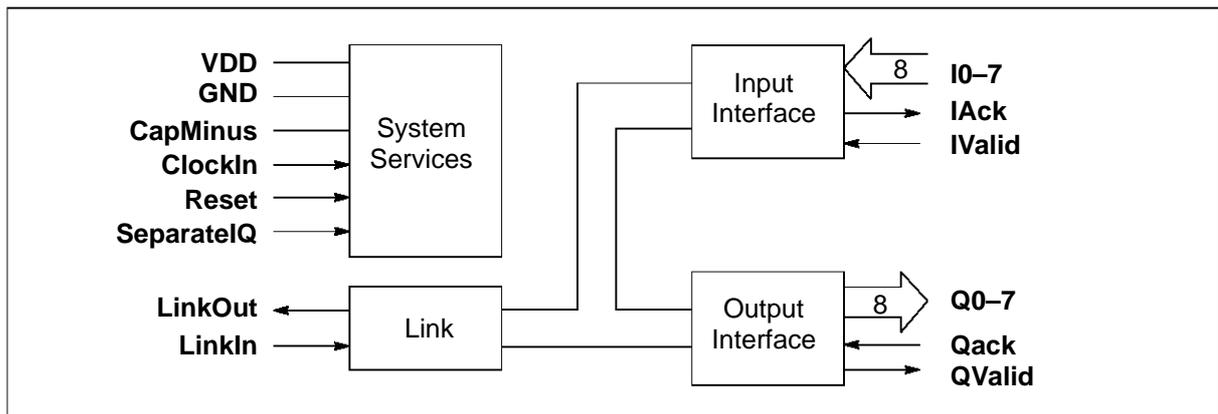
Figure 1.1 IMS C011E Mode 1 block diagram
