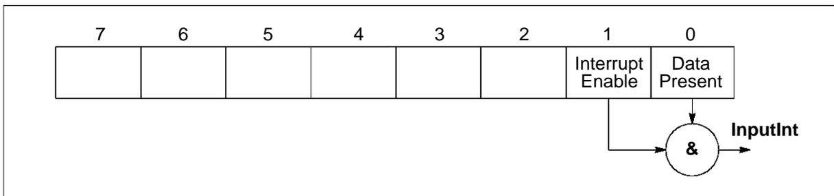
Figure 6.3 IMS C011E Mode 2 input status register
