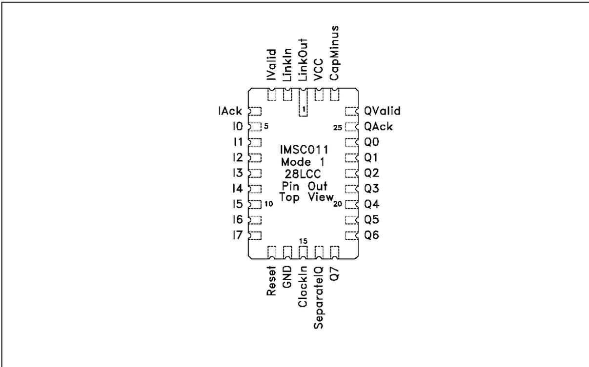
Figure 8.4 IMS C011E Mode 1 28 pin LCC package pinout
