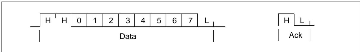
Figure 4.1 IMS C011E link data and acknowledge packets
