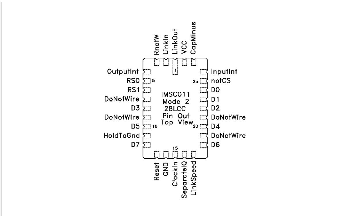
Figure 8.5 IMS C011E Mode 2 28 pin LCC package pinout
