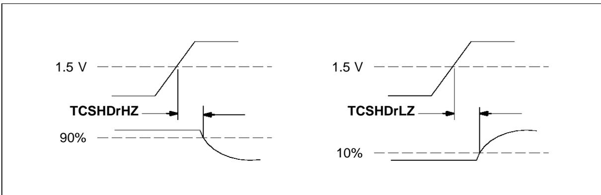
Figure 7.4 IMS C011E tristate timing relative to notCS
