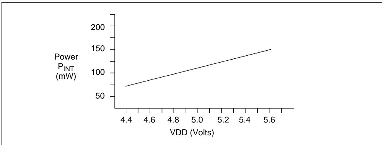
Figure 7.6 IMS C011E internal power dissipation vs VDD
