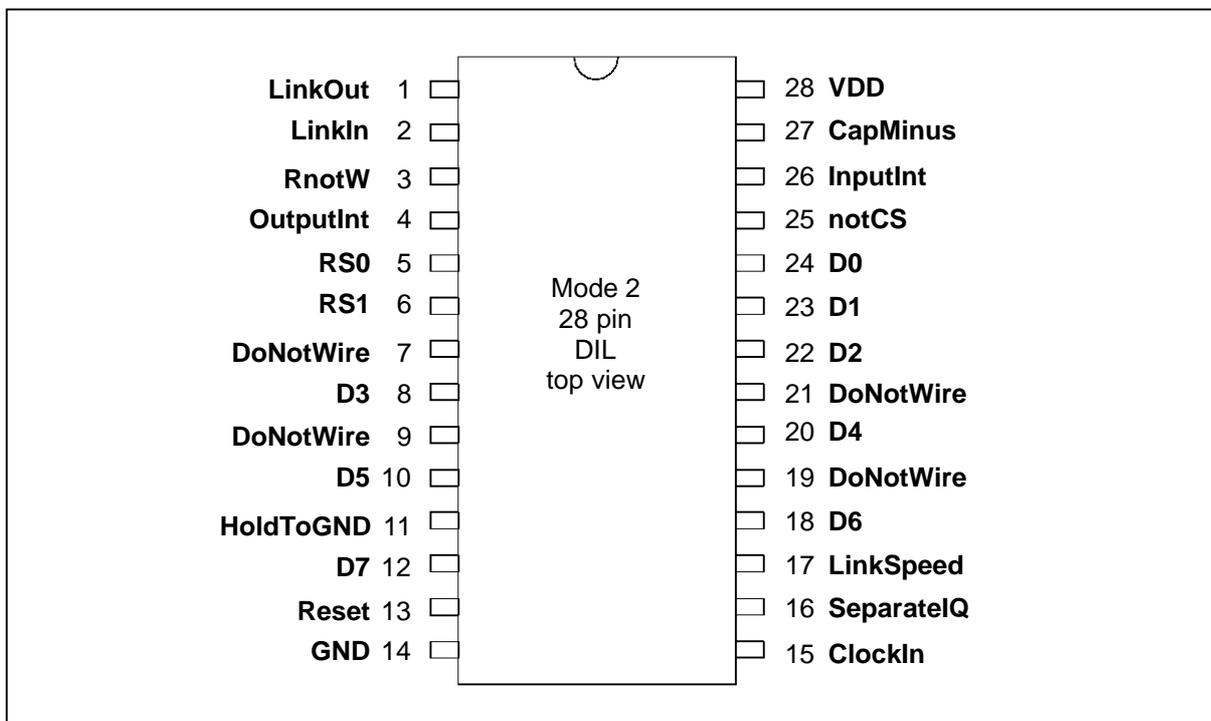
Figure 8.2 IMS C011E **Mode 2** 28 pin DIL package pinout
