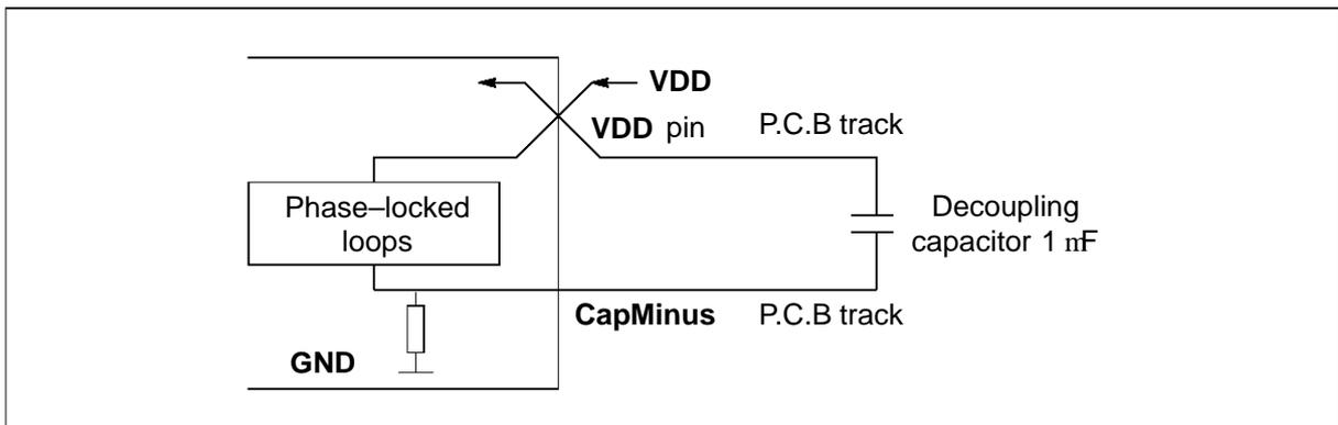
Figure 3.1 Recommended PLL decoupling
