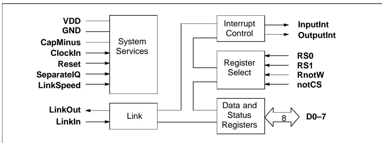
Figure 1.2 IMS C011E Mode 2 block diagram
