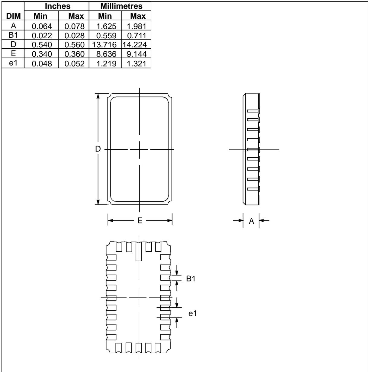
Figure 8.6 28 pin leadless chip carrier package dimensions
